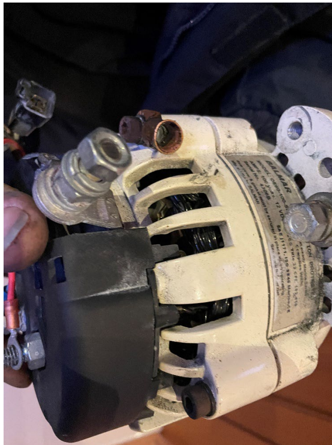
Fig. 6: The wiring inside the alternator should be a bright copper colour. The copper fitting at the top of the picture is where the temperature sensor is attached.
